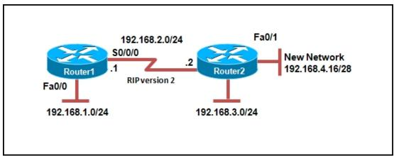
Refer to the exhibit. Router1 and Router2 are both running RIPv2 with autosummarization disabled. Which subnet mask will Router1 associate with network 192.168.4.16/28?
