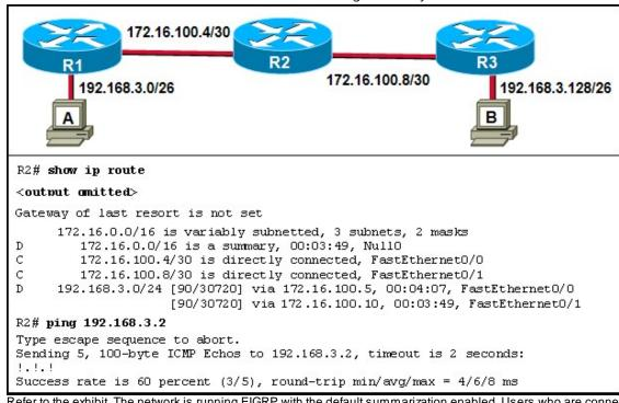
Refer to the exhibit. The network is running EIGRP with the default summarization enabled. Users who are connected to both R1 and R3 are complaining of intermittent connectivity. What should be done to solve this problem?
