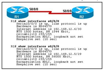
Refer to the exhibit. R1 and R2 are connected via serial interfaces. Both interfaces show that there is Layer 2 connectivity between the more than the connectivity between the two interfaces are unsuccessful. What is the conse of this connectivity between the two interfaces are unsuccessful. What is the consecutive that CDP is operational; however, pings between the two interfaces are unsuccessful. What is the connectivity between the two interfaces are unsuccessful.
