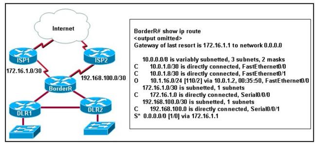
Refer to the exhibit. Internet access is crucial for the company network shown. Internet access is provided by two ISPs. ISP1 is the primary provider and ISP2 is the backup provider. The network administrator configures BorderR as the border router so that in normal operations, all Internet traffic goes through ISP1. However, if the link to ISP1 fails, then BorderR will automatically forward Internet traffic to ISP2. The administrator configures two default routes:
