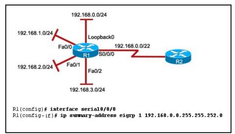
Refer to the exhibit. All routers are configured to use the EIGRP routing protocol, and the network administrator has configured the serial interface with the displayed commands. Which summary route will show in the routing table of R1 as a result of these commands?
