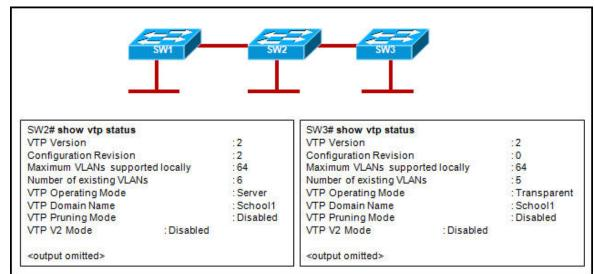
Refer to the exhibit. A network administrator noticed that the VLAN configuration changes at SW2 did not propagate to SW3. On the basis of the partial output of the **show vtp status** command, what is the possible cause of the problem?
