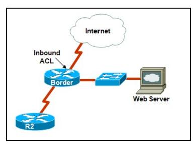
Refer to the exhibit. An enterprise web server has a private IP address. To allow access to the web server from external users, a static NAT statement is configured on the Border router. In an attempt to manage traffic that is bound for the server, the network administrator creates an inbound ACL on the outside NAT interface of the router. What address will be used in the ACL as the destination IP address?
