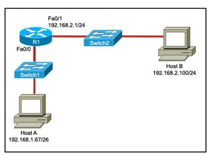
Refer to the exhibit. Which IP address can be assigned to the Fa0/0 interface of R1 to enable host A to access host B?
